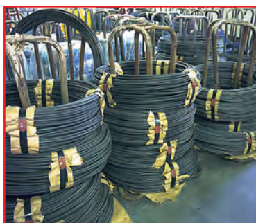
Material comes from the mill in large coils...which subsequently will be fed into cold-headers and formed into bolts.
